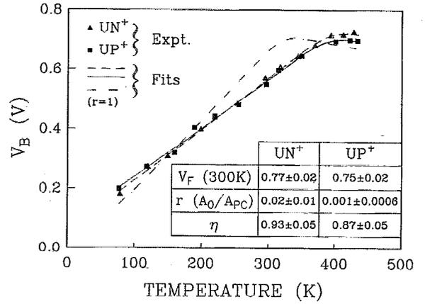
FIG. 2. The measured barrier height  $V_B(T)$ , in air, of  $UN^+$  (triangles) and  $UP^+$  (squares) samples as a function of temperature from Ref. 3. The solid ( $UN^+$ ) and dashed ( $UP^+$ ) lines are least-square fits to a current-transport equation with one pinning level ( $V_F$ ). The obtained values of  $V_F$ ,  $r$ , and  $\eta$  are shown in the inset. The dot-dashed line is a least-squares fit for the  $UN^+$  sample with  $r=1$ .
