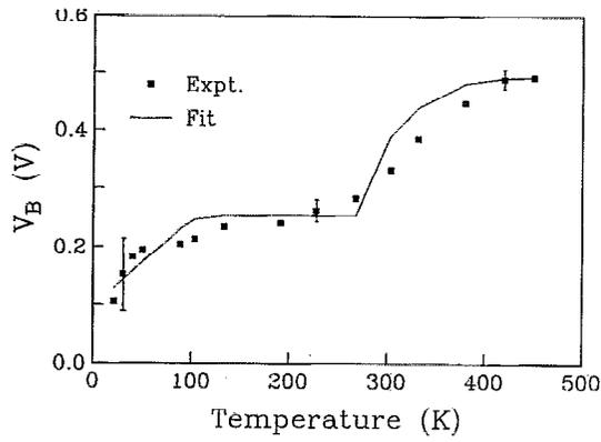
FIG. 1. The measured barrier height  $V_B(T)$ , in air, of a  $UP^+$  sample as a function of temperature. Representative error bars are shown. The solid line is least-square fit to Eqs. (2) and (4).
